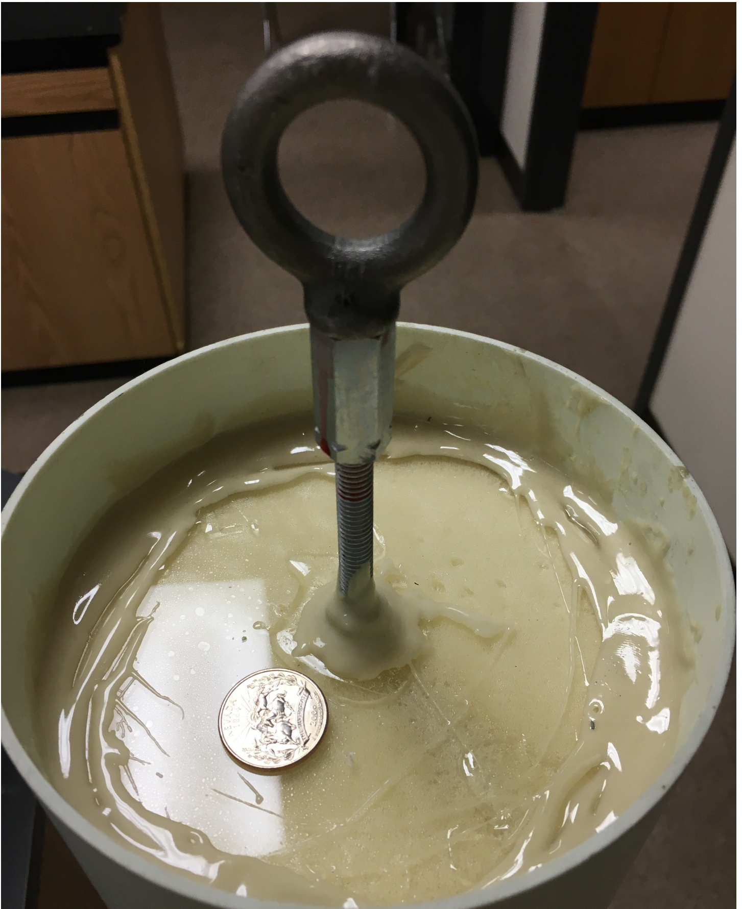
Left: Attachment point of the nose cone. A 5/16"-18 coupler joins the threaded rod and the eyebolt; heat locking threadlock is used to ensure a tight fit that will not unscrew due to vibrations (a swivel will also be used to prevent unscrewing the eyebolt).
