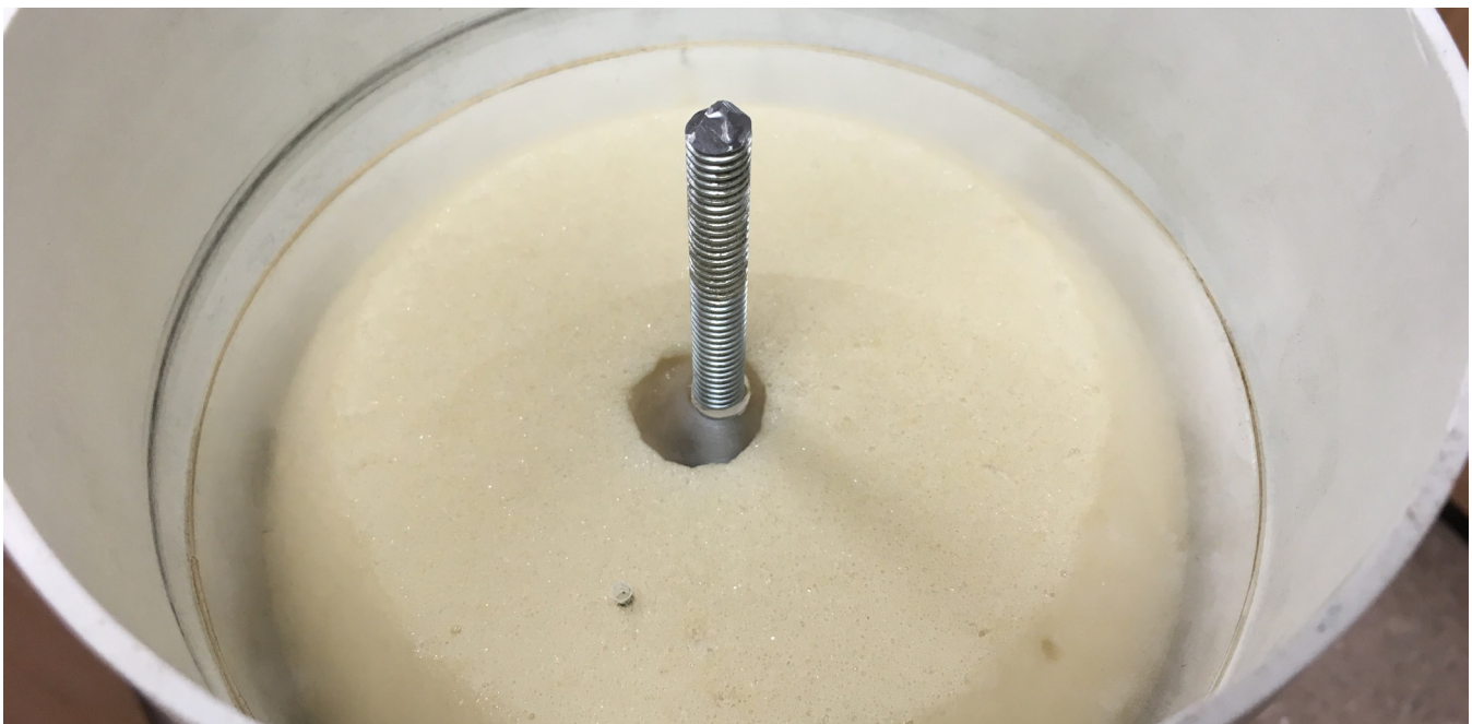
Top left: Schematic of the nose cone, complete with 5/16"-18 threaded rod core and several sealed bulkheads. The space is filled with 5:1 expanding foam for rigidity. Top Right: The alignment plate just below the nose cone coupler mount; epoxy joins the coupler to the nose cone. Below: Aft of the nose cone prior to eyebolt installation.
