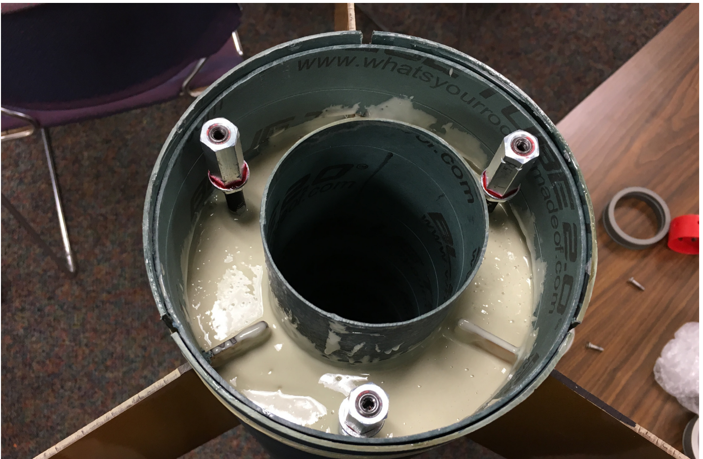
The motor section slid into place and filled with epoxy to secure the motor mount tube to the rocket.
